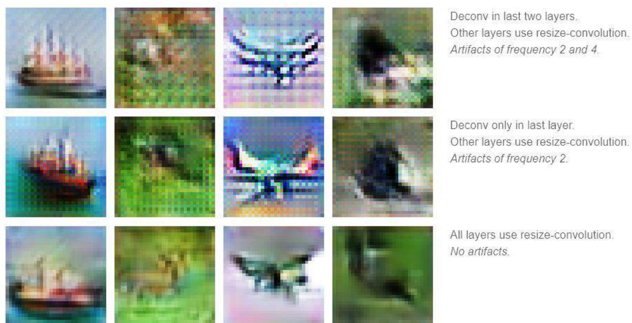
Figure 14. Examples of checkerboard artifacts produced by image deconvolution with and without corrective measures, reproduced from Odena et al. (2016).
